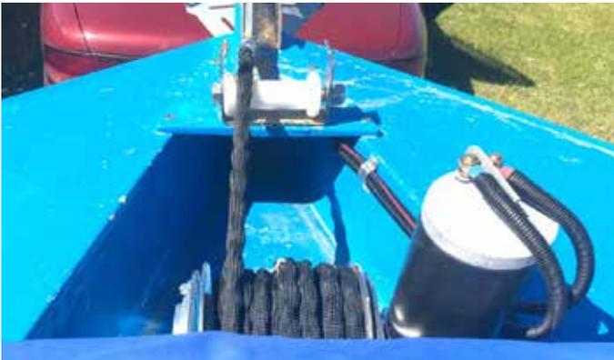
» Figure 1 The anchor drum and motor
