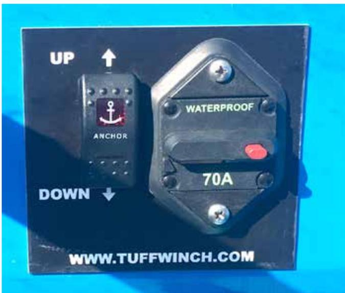
» Figure 2 Control panel for the anchor winch in the dashboard
